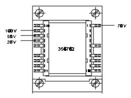
diagram 6 Switching the output voltage at the output transformers 356762
